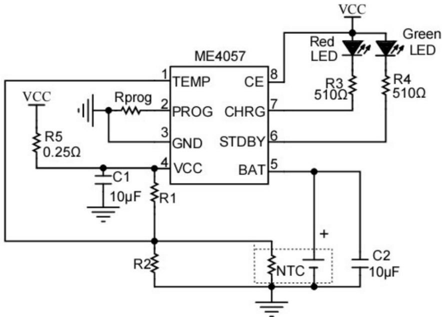
2. Suitable for 5V adapter and USB hybrid applications.
