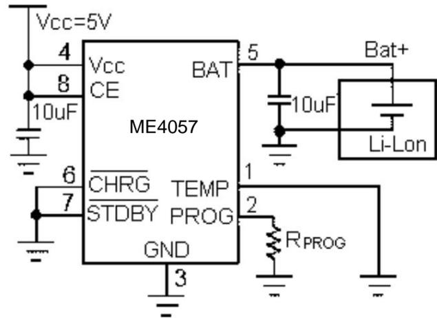
5. Add a power resistor to the input end to reduce chip power loss. When the red light is on, it means it is charging, and when the green light is on, it means the charging is stopped.
