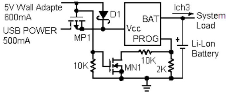
Figure 5: AC adapter and USB power supply combination
