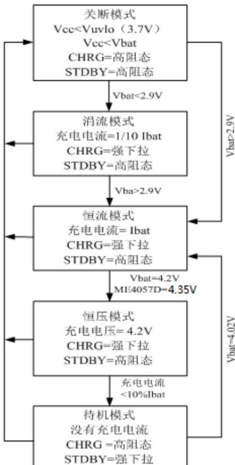
Figure 1: A typical charging cycle status diagram
