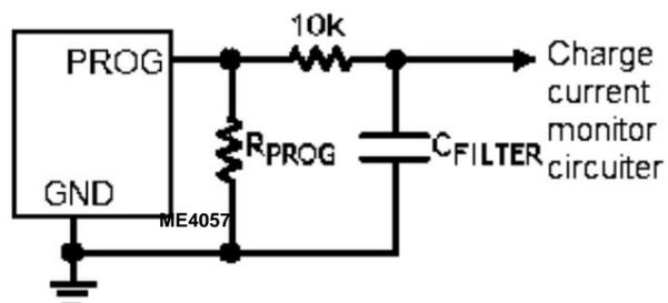
Figure 2: Capacitive load and filter circuit on isolated PROG pin
