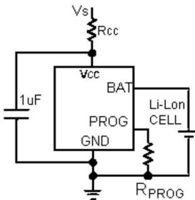
Figure 3: A circuit to increase charging current in thermal regulation mode
