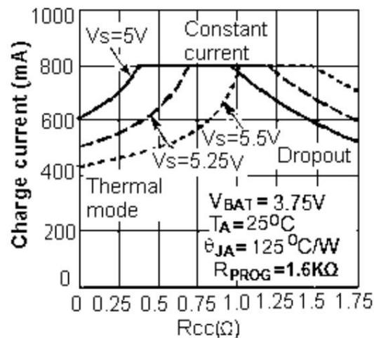
Figure 4: Charging current vs.  $R_{CC}$  relationship curve
