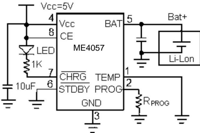
4. Suitable for applications that do not require charging status detection or battery
